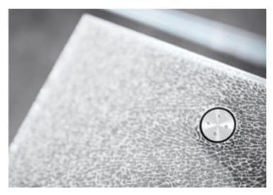
Righetti designs glass stairs made of triple tempered laminated glass to guarantee a high resistance against major impacts and to support heavy loads.
